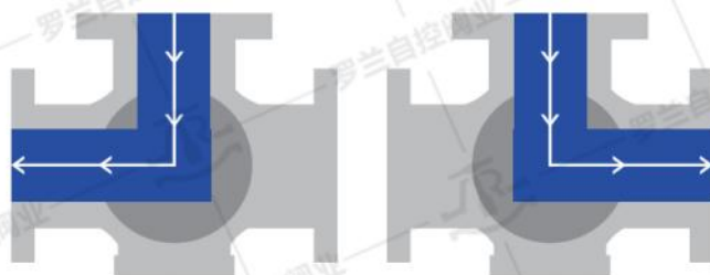
▶▶▶ L型通口三通球阀流向示意图
